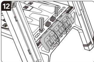
If desired, multiple units can be locked together side by side or end to end with the enclosed joiners.
