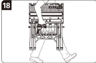
To carry Pegasus safely, only transport when folded, hold the table vertically and carry close to the body.
