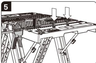
Push the clamping dogs into the desired holes on the table.
