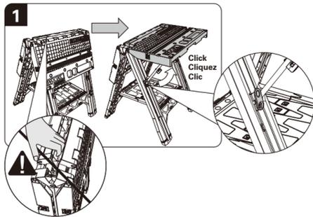
To use Pegasus as a work bench, open the legs fully and pull the table upward until latches "click" into place.
